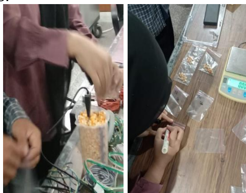
Gambar 3. Proses Kalibrasi Sensor Soil Moisture (SEN0308)
