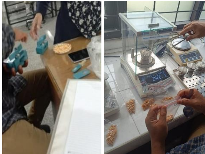
Gambar 4. Proses Kalibrasi Moisture Meter (G-WON)
